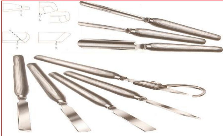
Figure 2.5: Types of wooden turning tools
