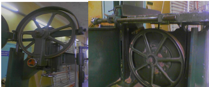
Picture 2. 4: Upper and Lower Drive Wheel
