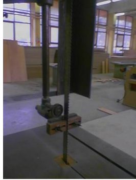
Figure 2. 5: Upper Guide Assembly
