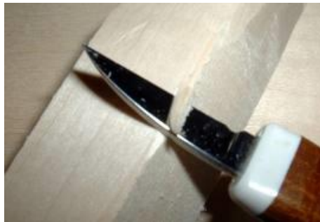
Picture1.63:Chamfer(Bevel)
