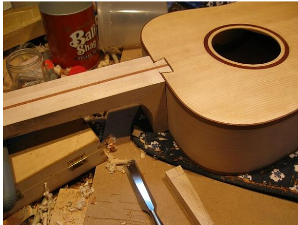
Picture1.77. Mounting the guitar neck to the body
