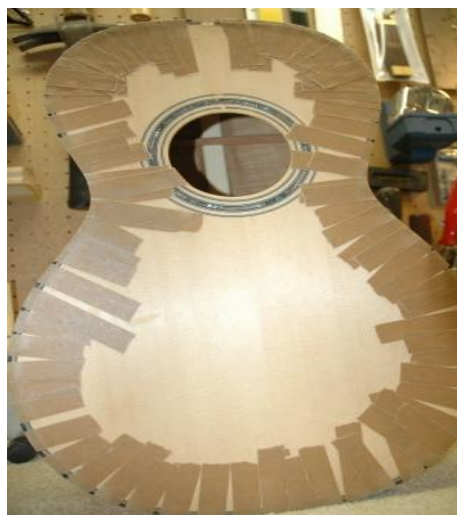
Picture 1.62: Sealing Guitar Body with Sellotape
