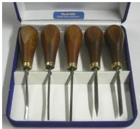
Picture1.48: Types of Straight Gouges
