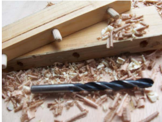
Picture1.75. Doweled edge joint
