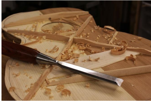
Picture1.46: Carving with Bevel Edge Chisel
