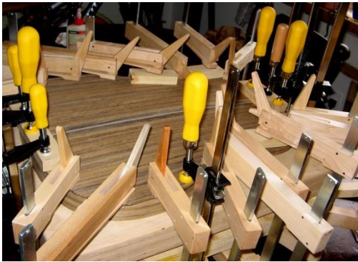
Picture1.58: Application of Eccentric Clamp in Making Guitar
