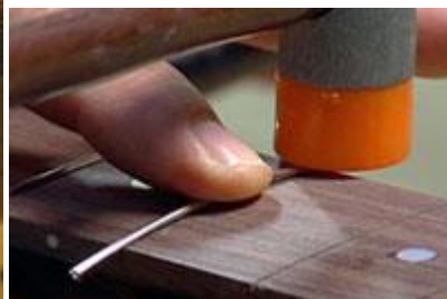
Picture1.51: Driving fret by use of plastic mallet
